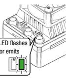
Move the throttle trigger to the end position
